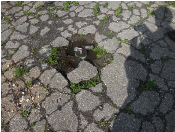
Monitoring well at Northern Area where ISCO testing is in process
